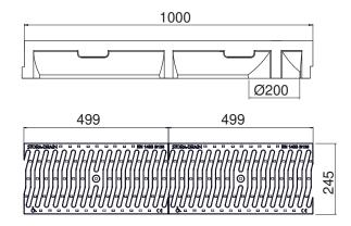
\* For channels SELF 200 / H=130 is necessary to buy STEPPED FALL to connect channels with SUMP UNIT.
